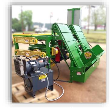
The Morgan Double Notcher manufactured by Sawmill Supplies and Equipment is designed for 4-way entry pallet stringers.
