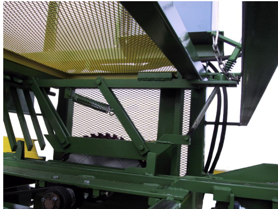
Adjustable spring loaded hold down system standard on all models.
