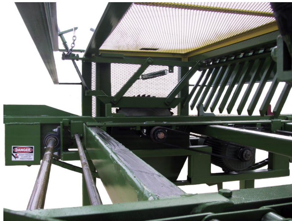
Adjustable spring loaded hold down system standard on all models.
